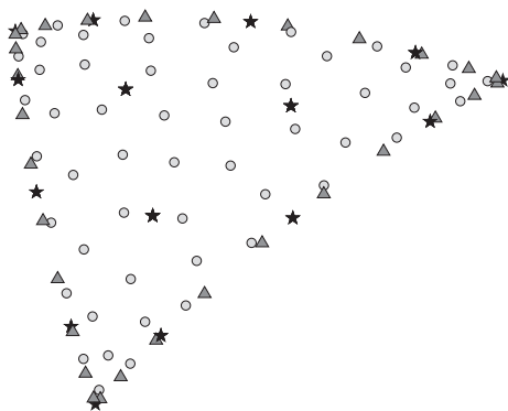
Fig. 3. Illustration of the cubature (circles) and Gaussian quadrature nodes (triangles) for N = 4 which results in N^c = 18 and N^g = 10 as well as N_p = 10 computational points (stars).
